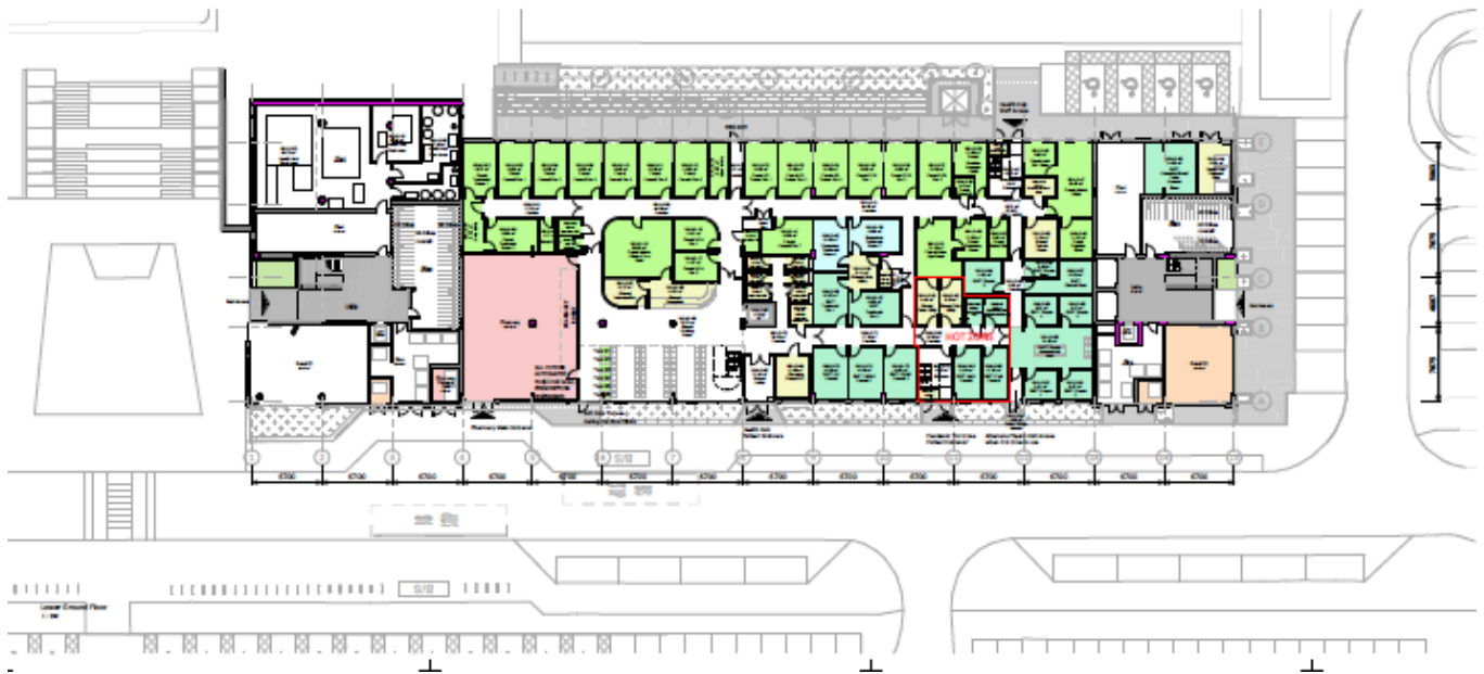
Image 5 - Lower Ground floor Primary care accommodation - Primary care shown in Green, Pharmacy space in pink. Community and sessional space is shown in blue
